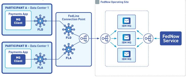
The application-to-application flow shown above supports an asynchronous messaging-based paradigm, implemented using IBM MQ. The FedNow Service hosts a cluster of IBM MQ queue managers, and the payment applications operated by Participants or their Service Providers interact directly with the queue managers to put and get
